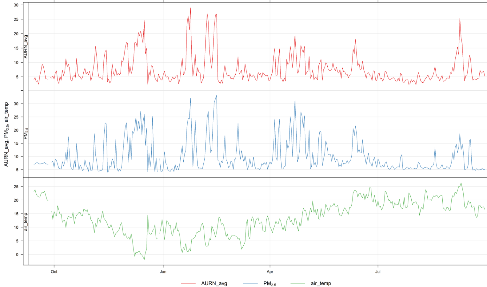
Figure A2.9: Time series plot of daily mean PM 2.5 concentrations (µg/m 3 ) at Z1083 (blue), average AURN PM 2.5 concentrations (µg/m 3 ) (red) and temperature (at Zephyr) (°C) (green), September 2022 to September 2023
