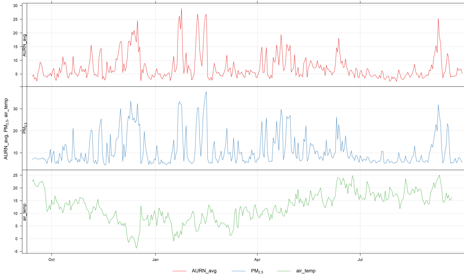
Figure A2.5: Time series plot of daily mean PM 2.5 concentrations (µg/m 3 ) at Z1142 (blue), average AURN PM 2.5 concentrations (µg/m 3 ) (red) and temperature (at Zephyr) (°C) (green), September 2022 to September 2023
